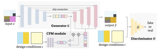
Figure 8: Model architecture of the color recommender in De-Stijl, consisting of a generator G connected by skip connections along with a Condition Feature Modulation (CFM) module and a discriminator D. Taking the image layer  $L_i^p$  as an example (input and output for other layers are shown in Figure 7), given the input x, the generator will output the recommended color palette  $\hat{y}$  according to the design conditions c.
