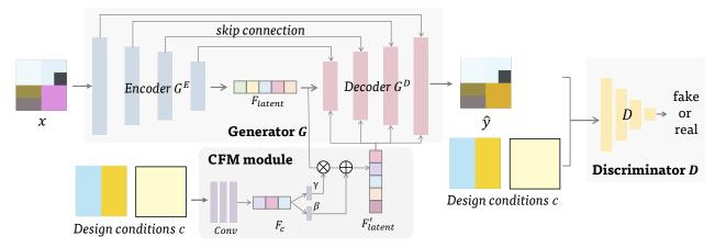
Figure 13: Model architecture of the color recommender in De-Stijl, consisting of a generator G connected by skip connections along with a Condition Feature Modulation (CFM) module and a discriminator D. Taking the image layer  $L_i^p$  as an example, given the input x, the generator will output the recommended color palette  $\hat{y}$  according to the design conditions c.
